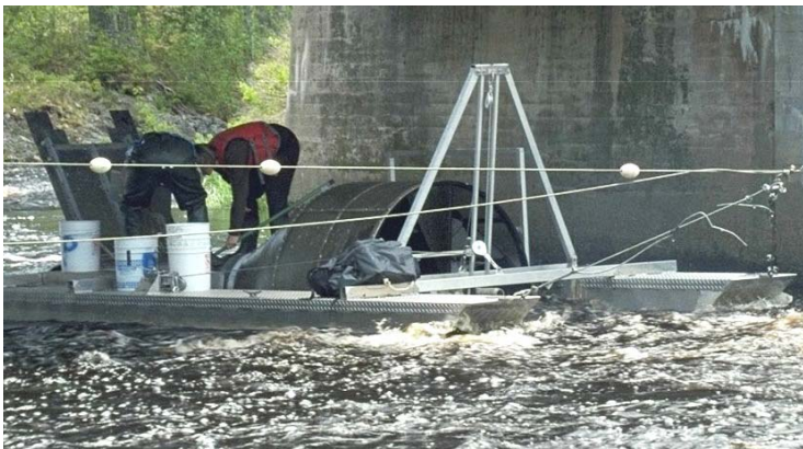
Among other things, NEST uses its rotary screw traps as a platform to collect smolts for telemetry studies.
