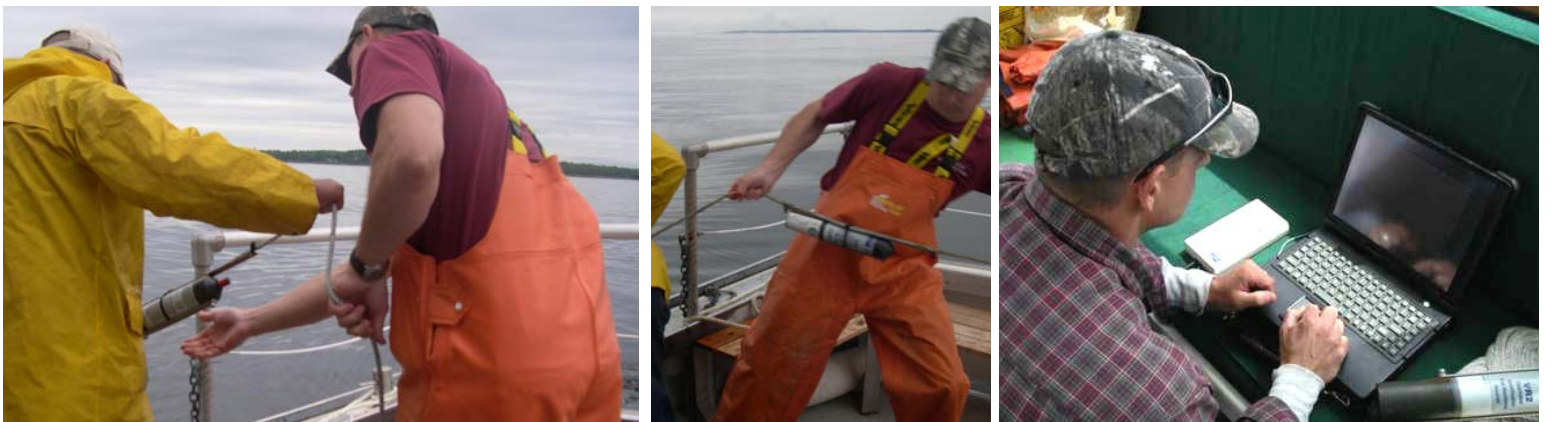
Vessel contractor Michael Ormsby and NEST contractor Graham Goulette retrieve a VR2 receiver from an array in Penboscot Bay. After retrieval, data collected by the VR2 is downloaded (right) and used to gain a better understanding of emigrating smolt behavior and mortality.
