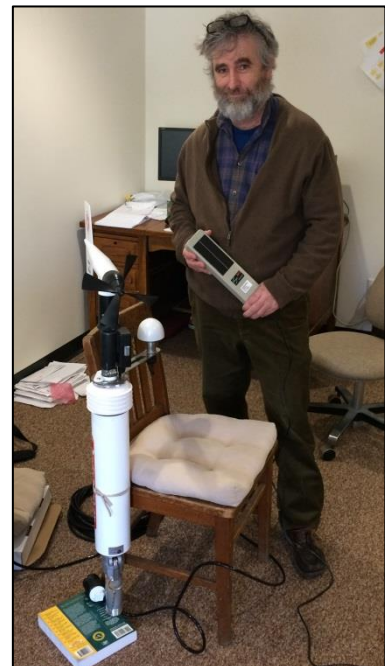
Jim Manning holds the satellite transmitter for a shipboard weather station undergoing testing in his office. The transmitter will be mounted on the fishing vessel's wheelhouse roof.
