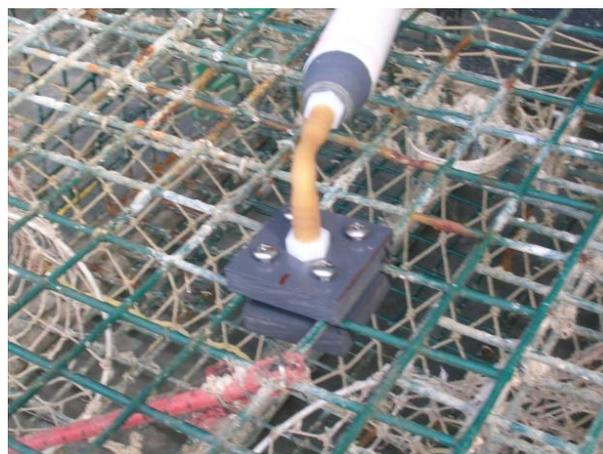
Fig 4. Seahorse current-meter attachment to lobster trap.
