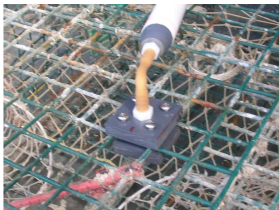
Fig 4. Seahorse current-meter attachment to lobster trap.
