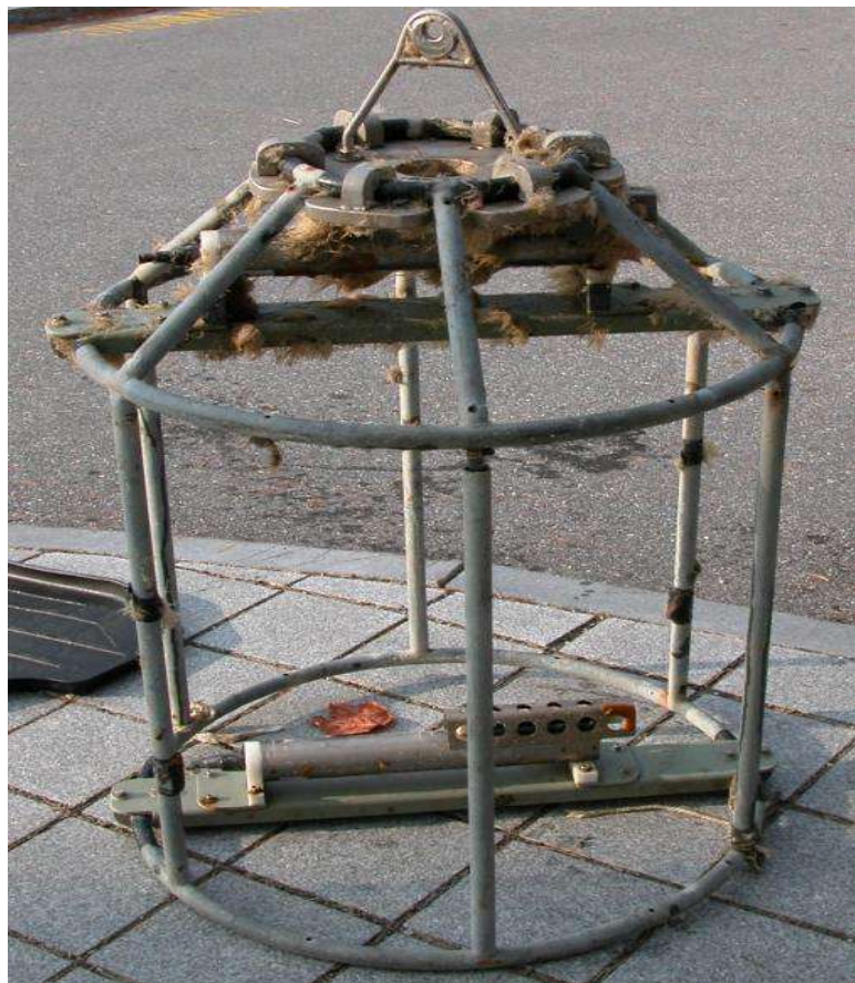
Figure 3. Seabird Microcats secured to frame after two months in Quohog Bay.
