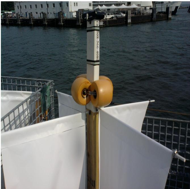
below) holds the most promise in replacing the Rachel as our standard surface drifter. While the first Eddie prototype failed after a few days, the 2<sup>nd</sup> has been reporting regularly for 3 weeks. Not only is this drifter a bit more environmentally friendly, it is much easier to make and should cost hundreds less. More info on these alternative models is posted with photos on the “drifter design and technology” link on the drifter website <http://www.nefsc.noaa.gov/drifter>
